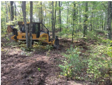
Root rake dozer used to scarify the ground to improve acorn regeneration. Photo by WI DNR
