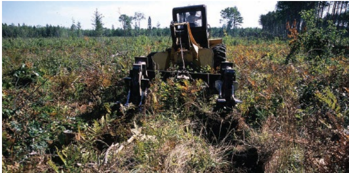
Leno Scarifier in Action.
